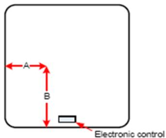
If your intent is to bring a conduit and power wires up under the spa we suggest that it enter the spa cavity in the front, left corner; 6" (15cm) Dimension A in from the left and 6" (15cm) Dimension B up from the front. See A & B on the diagram below. This location will allow you to stay clear of spa pumps and other equipment while giving you a short and easy access to the left side of the spa pack, where the electrical entry hole and terminal block are located.
