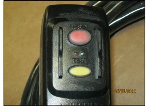
FAMILIARIZE yourself with the test procedure for the GFCI. TEST the GFCI upon every use of the spa.
